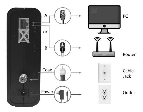
**Option A:** Direct Connection - If you are only connecting to one device, you can connect directly to the modem. Connect one end of the ethernet cable to the yellow LAN Port '1' on your modem, and the other end to an ethernet LAN port on the device you want to connect.
